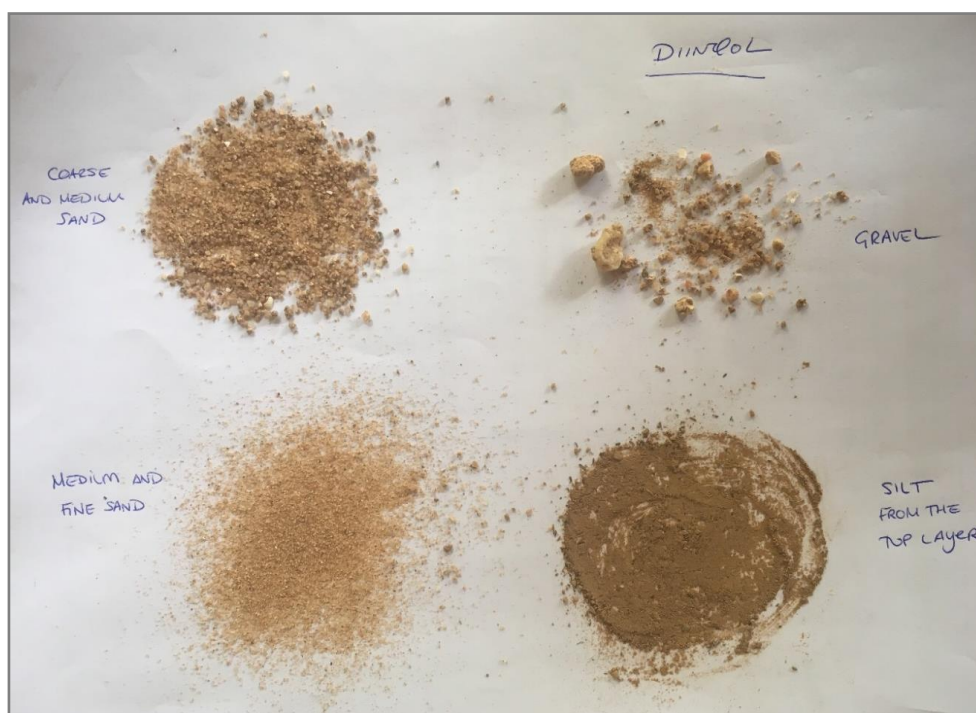
Diinqal sand sample taken at a depth 30cm in the dam throwback and the top dry silt layer.
