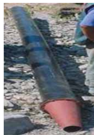
Fig Penstock pipe made of PVC pipe with nozzle
