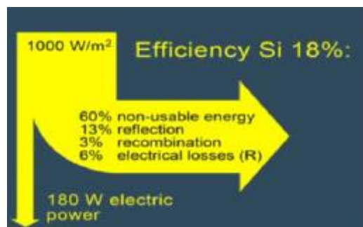
Figure 6: The efficiency of a 180W solar panel with an 18% efficiency rating 9
