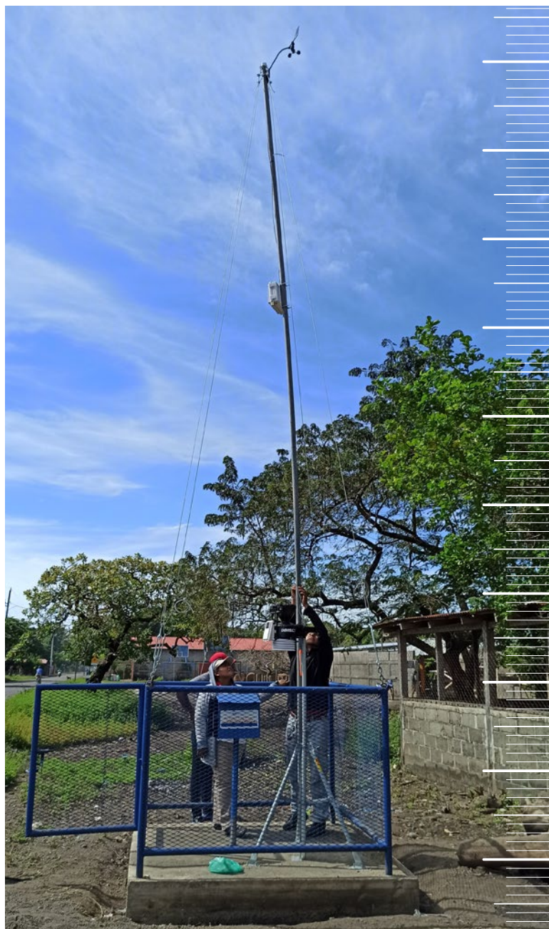
The technical team from INETER installing the new communal weather station in Mechapa, Chinandega, Nicaragua © Felix Rugama, Plan International
