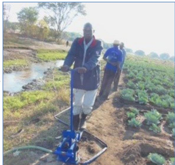
*A treadle pump in action in Zambia. The pump helps reduce the reliance on rain-fed agriculture.*
